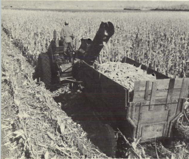
Corn-picking machines handle 12-15 acres a day. An efficient crop, corn has a high yield per acre.
