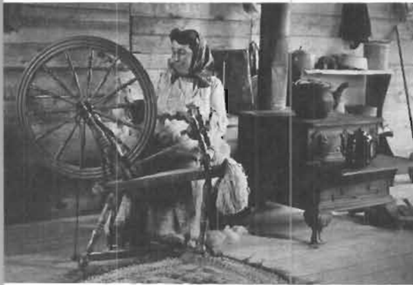
Interior of the Laverdure summer kitchen at Valcourt d'Ely showing a woman drawing out and twisting wool fiber into thread with the aid of a foot-driven spinning wheel. (Courtesy Department of Media Services, Dimond Library, University of New Hampshire.)
